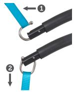
Patented Ergolet sling hooks on the spreader bar. Sling attachment: a minimum of downward pressure locks the sling hook; pull upwards to unlock sling hook.
