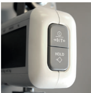
On/Off/Zero/Tare and Hold buttons
