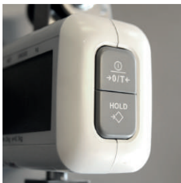
On/Off/Zero/Tare and Hold buttons
